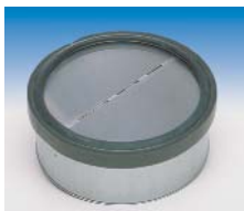
Backdraft damper with spring return prevents cold air from entering when fan is not in use.
